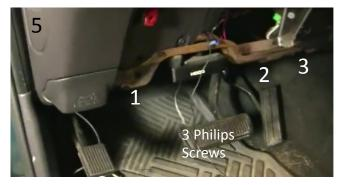
6. Unbolt emergency brake pedal lever (or kick plate covering the emergency brake on some models) to facilitate wire routing thru the rubber boot between the door and the body of the truck. To do this, remove the 3 bolts around the brake peal lever. One is on the side (6.1) and the other two back on the firewall (6.2).
